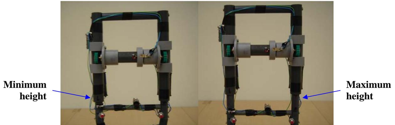
Figure 10: Walking crutch at its minimum height (left) and maximum height (right)
