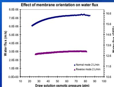
Fig 5: Graph of effect of membrane orientation on the water flux
