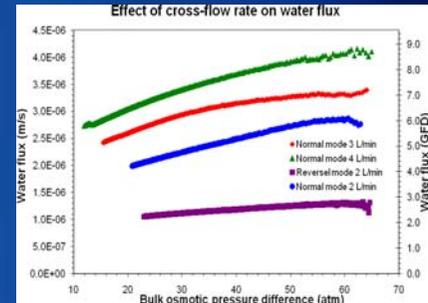
Fig 6: Graph of effect of flow rate on the water flux
