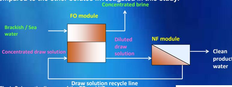
Fig 1: Schematic diagram of the FO and NF process
