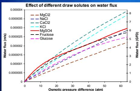
Fig 4: Graph of effect of different draw solutes on the water flux (m/s)
