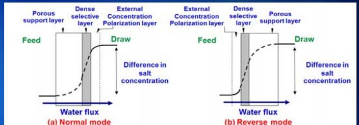
Fig 3: Schematic diagram of the effect of membrane orientation on FO transport phenomenon
