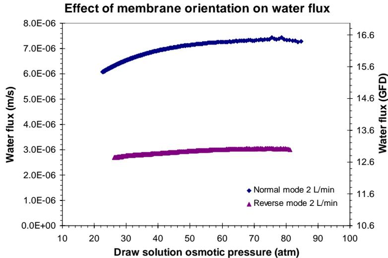
Figure 5: Graph of effect of membrane orientation on the water flux (software: Microsoft Excel 2003)
