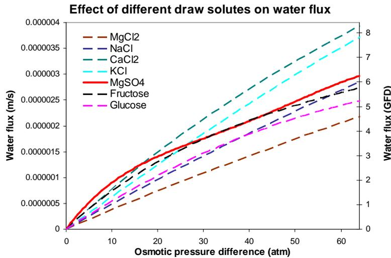
Figure 4: Graph of effect of different draw solutes on the water flux (m/s) (software: Microsoft Excel 2003)
