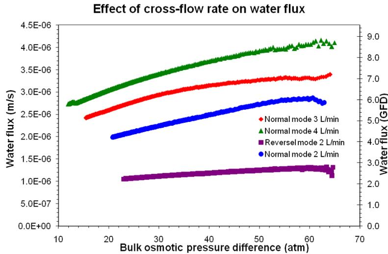
Figure 6: Graph of effect of flow rate on the water flux (software: Microsoft Excel 2003)
