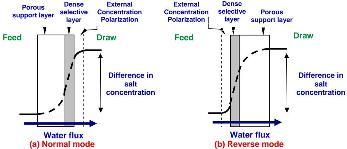
Figure 3: Schematic diagram of the effect of membrane orientation on FO transport phenomenon (software: Microsoft PowerPoint 2003)
