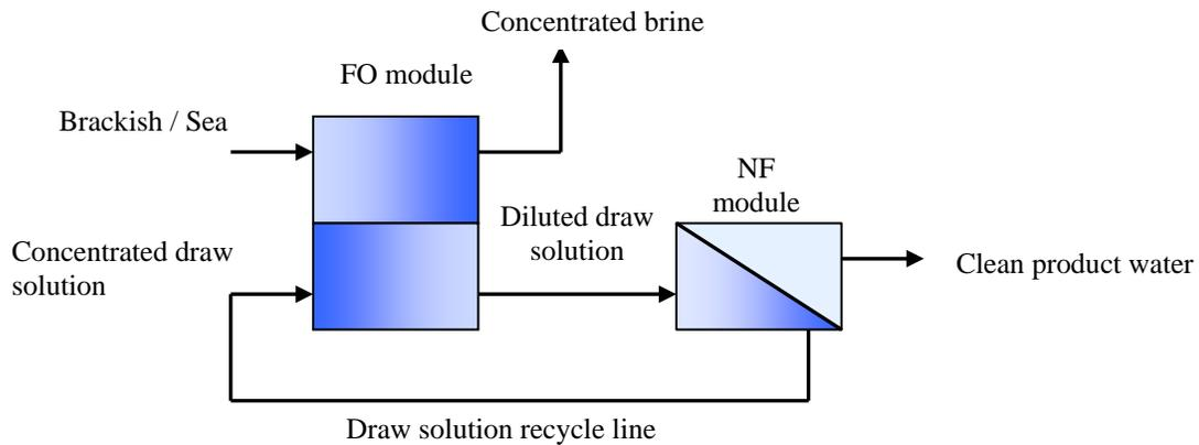
Figure 1: Schematic diagram of the FO and NF process (software: Microsoft Word 2003)
