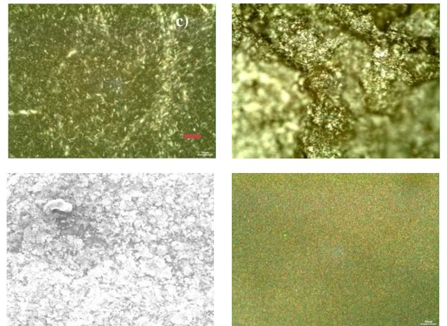
Figure 6. Microscope Images (Nikon camscope) of device surface morphology. Voids can be clearly seen in a) annealed polymer layer as well as b) annealed silver layer. c) The rough texture of the silver with polymer contact in contrast with d) unannealed polymer surface in
