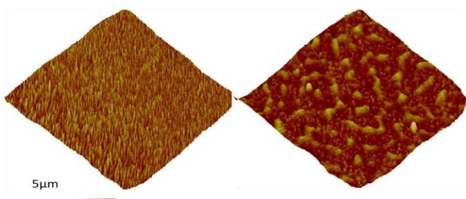
Figure 4. AFM height images of polymer composite (PCBM:P3HT concentration= 1:1) surface morphology before (left) and after (right) thermal annealing. A more regular and rougher surface is obtained after heat treatment, indicating greater blending with carbon nanotubes. Captured surface area is 5 μm×5 μm.
