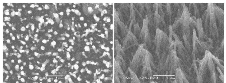
Figure 3. SEM images of carbon nanotubes a) before and b) after the functionalization and deposition of P3HT:PCBM layer. The clump aggregates may imply the attachment of polymer particles to oxidized tips of CNTs via van der Waals.
