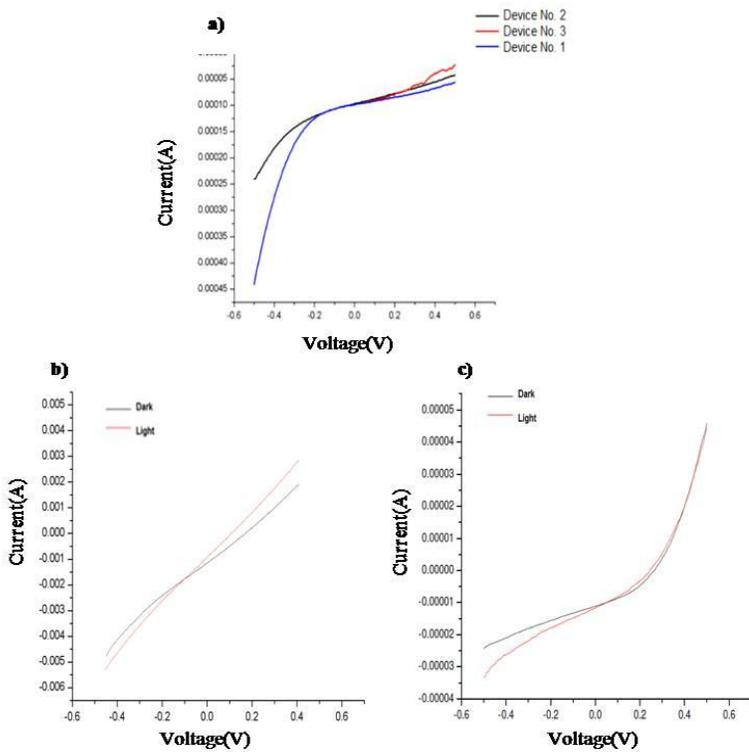
Figure 5. a) I-V characteristic curves of devices measured under illumination. The conditions are: Device 2 (5 mins), Device 3 (10 mins) at 110°C and Device 1 (unannealed). b) Device 6 and c) Device 7 under illumination respectively.
