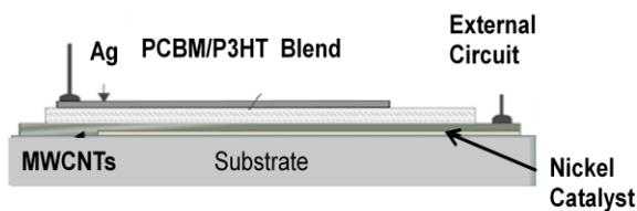
Figure 1. Schematic layout of fabricated organic polymer (PCBM-P3HT) solar cell incorporating carbon nanotubes and silver metal as electrodes. Ref [5]
