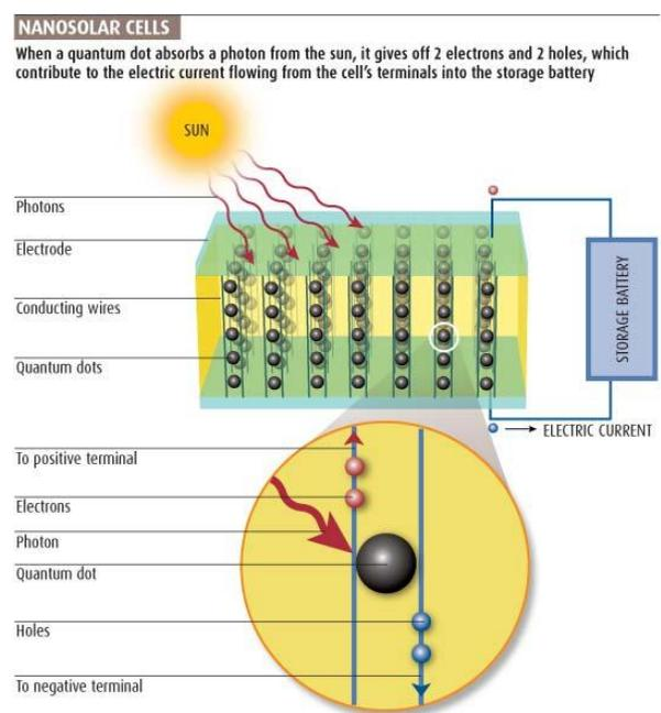
Figure 2. Diagram illustrating operational principle of polymer solar cell, including the propagation of charge carriers under illumination and transport to electrodes. The quantum dot in the figure would theoretically refer to some P3HT particles in this experimental, attached to carbon nanotubes. Ref [4]
