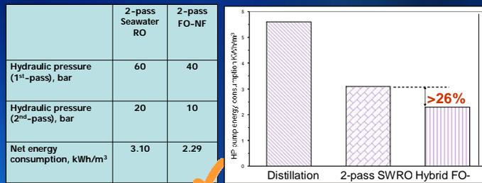
Fig 5: Comparison of energy consumption of RO and FO-NF
