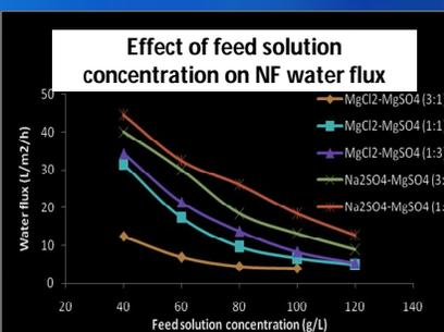
Fig 3: Graph of NF water flux against feed solution concentration
