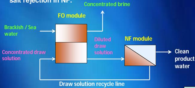
Fig 1: Schematic diagram of the FO and NF process
