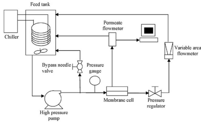
Fig 3: Schematic diagram of the Nano-filtration experimental Set-up (software: Microsoft Word 2003)
