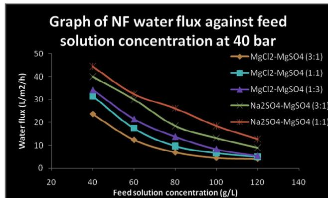
Fig 6: Graph of NF water flux against feed solution concentration at 40 bar (software: Microsoft Excel 2003)
