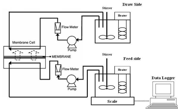
*Fig 2: Schematic diagram of the Forward osmosis experimental Set-up (software: Microsoft Word 2003)*
