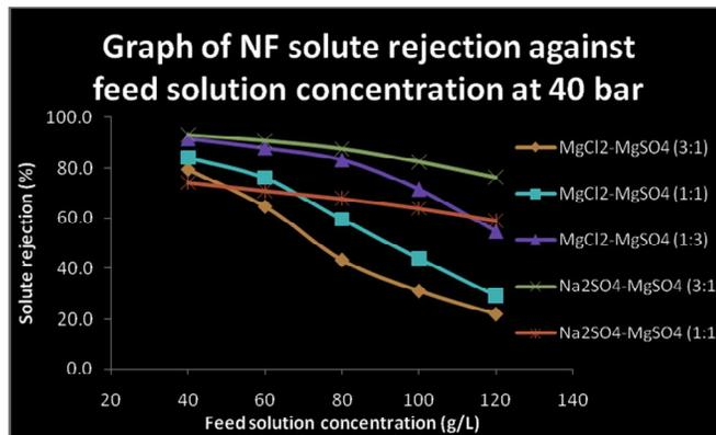
Fig 7: Graph of NF solute rejection against feed solution concentration at 40 bar (software: Microsoft Excel 2003)
