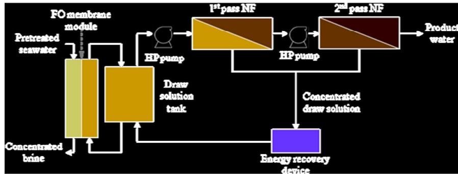
Fig 1: Schematic diagram of the FO-NF hybrid experimental Set-up (software: Microsoft Word 2003)
