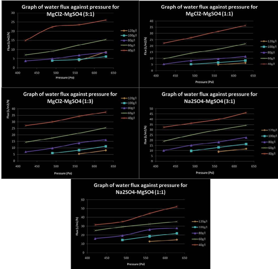
Fig 8: Graph of water flux against pressure for 8.1: MgCl<sub>2</sub>-MgSO<sub>4</sub> (3:1); 8.2: MgCl<sub>2</sub>-MgSO<sub>4</sub> (1:1); 8.3: MgCl<sub>2</sub>-MgSO<sub>4</sub>(1:3); 8.4: Na<sub>2</sub>SO<sub>4</sub>-MgSO<sub>4</sub> (3:1); 8.5: Na<sub>2</sub>SO<sub>4</sub>-MgSO<sub>4</sub> (1:1) (software: Microsoft Excel 2003)
