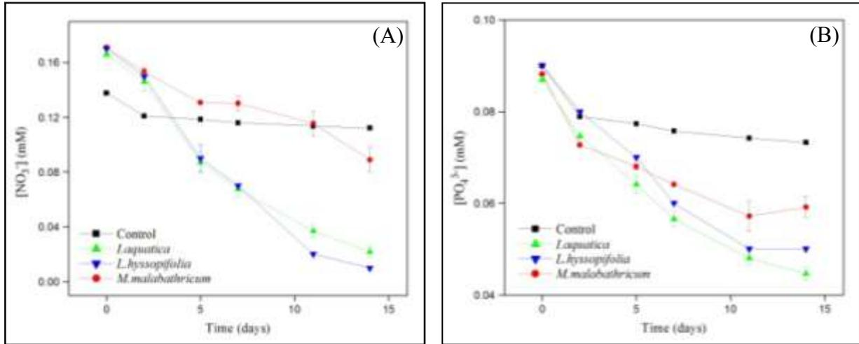
Figure 1. Kinetics of the removal of (A) nitrate and (B) phosphate by emergent aquatic macrophytes
