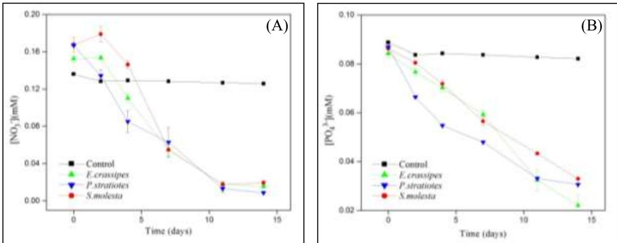
Figure 2. Kinetics of the removal of (A) nitrate and (B) phosphate by floating macrophytes
