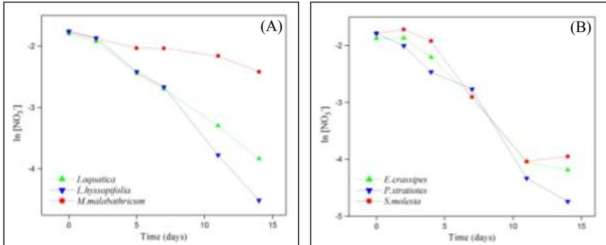
Figure 3. Kinetic analysis of nitrate removal by (A) emergent and (B) floating macrophytes
