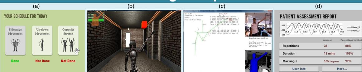
Fig. 2: Game Design and Interfaces: (a) Exercise Schedule UI (b) Game play UI (c) Kinect Outputs and Joint Angles Recording UI (d) Exercise Assessment Report UI [(a) and (d) are self-designed UI illustrations (b) and (c) are self-taken screenshots]
