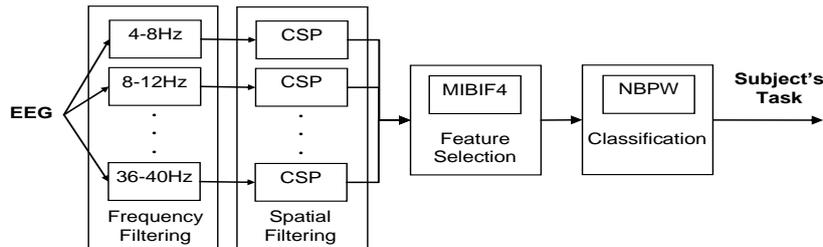
**Figure 2: Filter Bank Common Spatial Pattern Algorithm which performs 4 stages of signal processing and machine learning to decipher the subject's action from the EEG**
