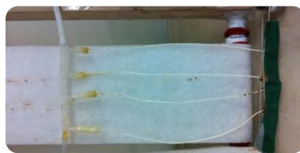
Figure 11. With mechanical cleaning using the self-designed wiping system—no fouling observed
