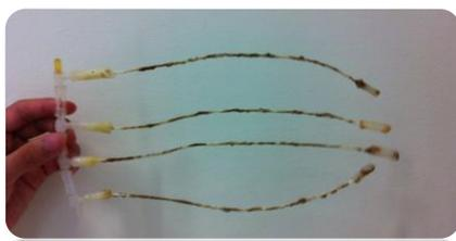
Figure 10. Control (without mechanical cleaning) – fouling observed
