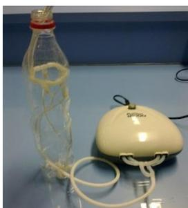
Hollow fibre membranes were placed in an enclosure (plastic bottle) and concentrated bubbling was provided by the air pump. The air bubbles will knock off the particles deposited on the hollow fibre membranes, thus reducing fouling.
