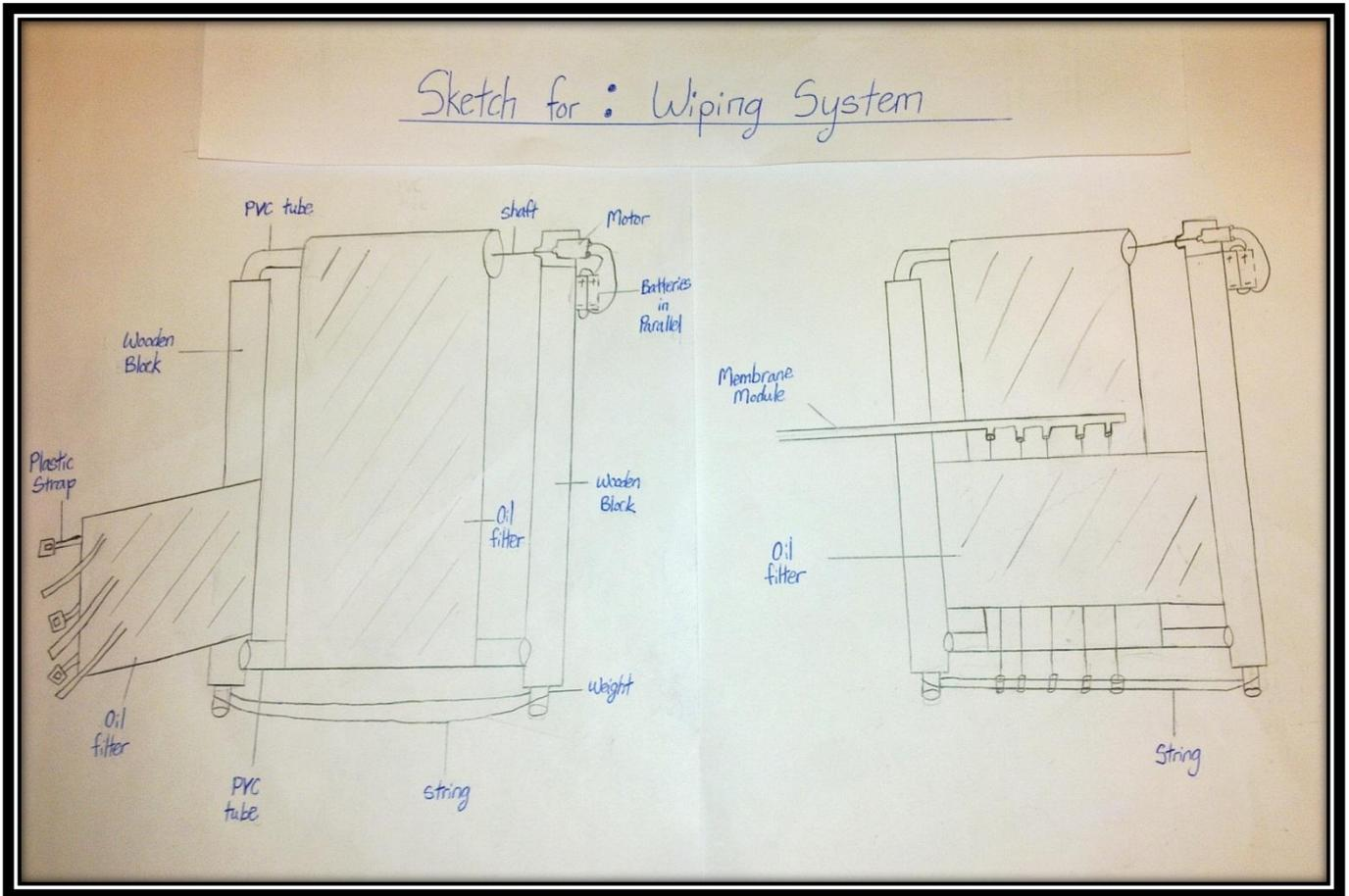
2) Use of mechanical cleaning (self-designed wiping system)
