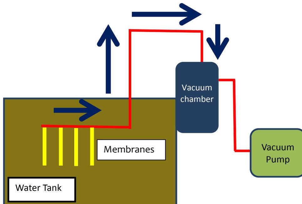
Figure 3. Experimental set-up to determine flux rate
